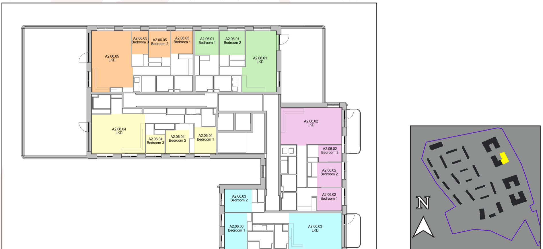
Figure 7.89: Floor plan of assessed building (L), Keyplan highlighting the assessed building (R).
