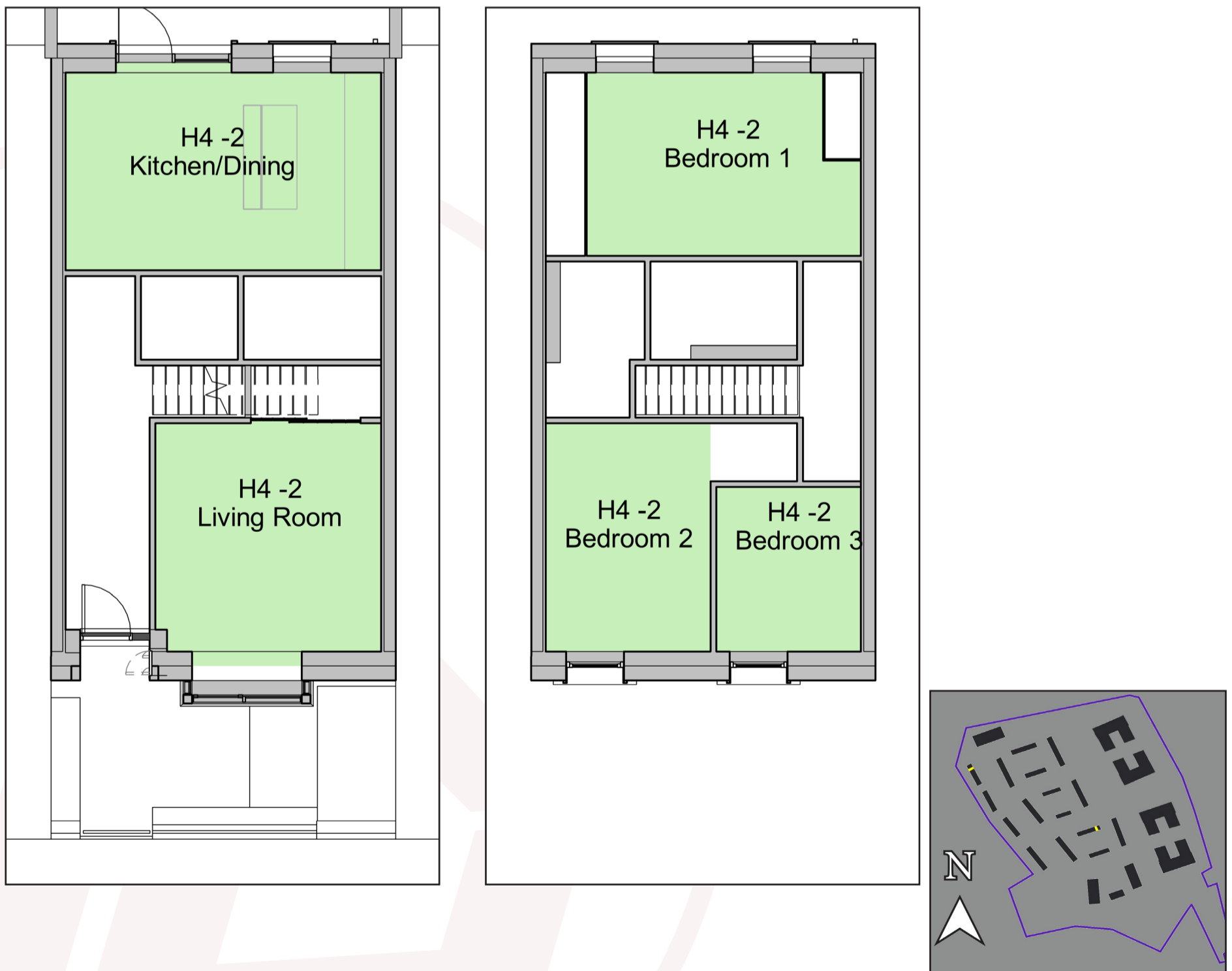
Figure 7.65: Floor plan of assessed building (L), Keyplan highlighting the assessed building (R).
